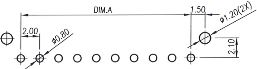
Recommended PCB Layout (Tolerance ± 0.05)
